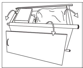
**STEP 1:** Lay down tank housing assembly (K) as shown above. Take off the door and take out all parts.
