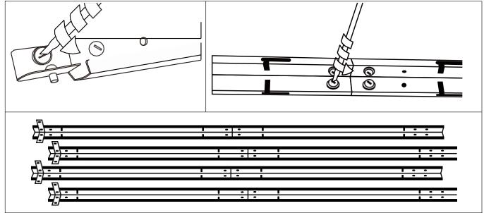
**STEP 3:** Unscrew 2pcs M5 screws and washers (BB) preassembled in Support Bar – Lower (F). Insert upper Support Bar (E) to lower Support Bar (F) and fix the connection using 2pcs screws and washers (BB). Repeat this step and connect other 3 sets of support bars.
