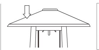
**STEP 5:** Place Reflector (A) on the Flame Screen (B) and fix the connection using 4 M5 CAP NUTS (AA).
