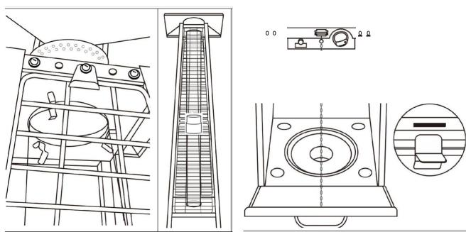
STEP 11: Assemble Lower Mesh Guard (D) STEP 12: Insert the feet of the door into the bottom and Upper Mesh Guard (C) in the front. Fix 4 slots. Attach the Chain (L) to the hook of the Burner Guard Fastening Plates to keep Upper Mesh Assembly (J) and close the door.
