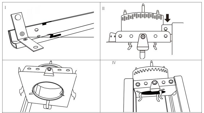
**STEP 4:** Attach Flame Screen (B) to the top of upper Support Bar (E) and fix the connection using 2 M5 screws and washers (See Figure  $\blacksquare$ ,  $\blacksquare$ ).
