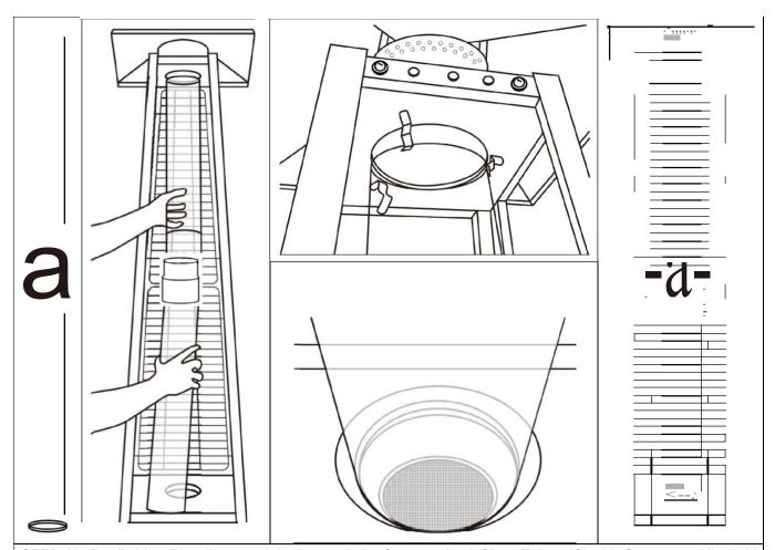
**STEP 10:** Put Rubber Ring (I) around the burner hole. Connect the 2 Glass Tubes (G) with Connector (H). Hold the whole glass tube assembly carefully. Insert the top end into the bottom hole of the Flame Screen as much as possible. Keep the whole glass tube assembly vertical and sit it on the Rubber Ring (1).
