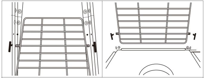
**STEP 7:** Insert 4 projecting ends of each lower Mesh Guard (D) into the seat slots of lower the Support Bar (F) as shown in picture. Fix all lower Mesh Guards (D) except the front side.
