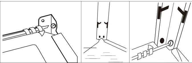
**STEP 6:** Unscrew 8 M5 Screws and Washers (BB) preassembled on top of tank housing assembly (K). Place the lower Support Bars to the top of the tank housing assembly. Make sure to match the top ends of the tank housing assembly with the slot of the lower Support Bar. Match the threaded hole and fix each connection with 2 M5 Screws and Washers (BB)
