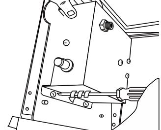
**STEP 2:** Keep the burner with the igniter side up. Fix the burner assembly (J) to tank housing using 4pcs M5 Screws and Washers (BB).
